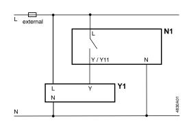
N1 = room thermostat Y1 = actuator SUA21/3P Y/Y11 = control signal OPEN L = phase N = neutral
